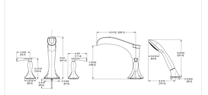
Ø1 Min to Ø1-1/2 Max. Deck Hole Openings
