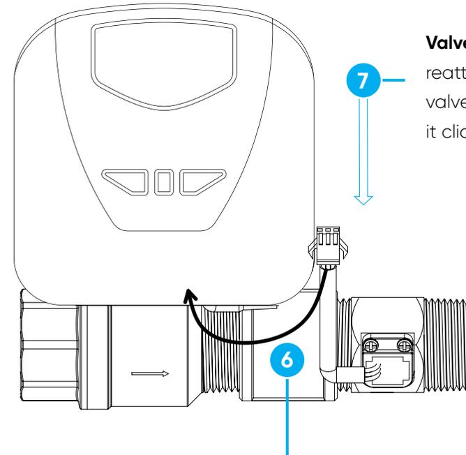
**Valve control head:** reattach to the shut-off valve by sliding on until it clicks into place.
