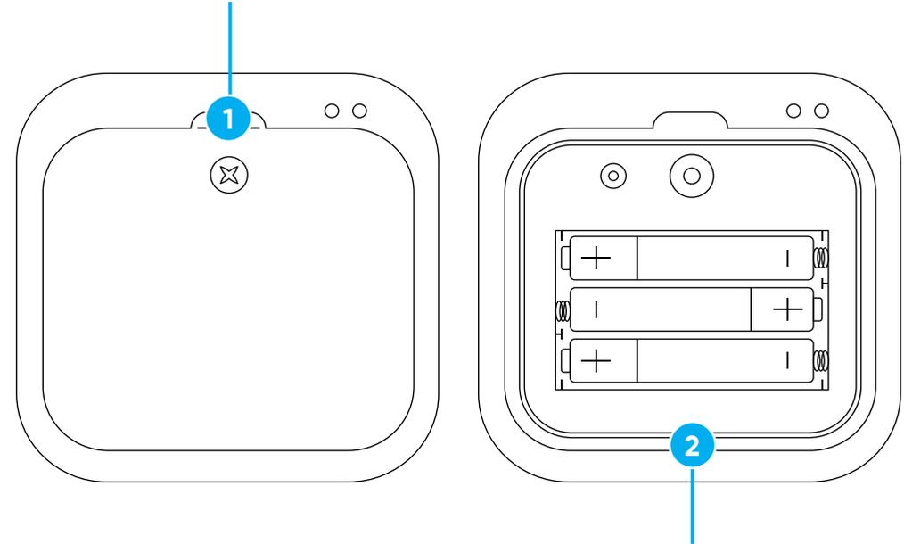
**AAA batteries:** install three batteries after temporarily removing battery door.
