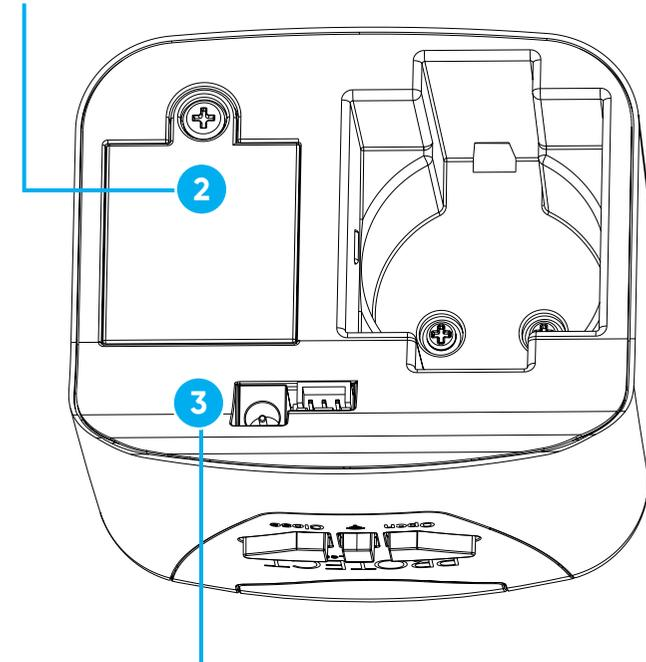
**9V Supply Cord Jack:** plug cord into outlet after insertion.
