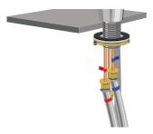
5. Attach the main supply lines to the braided water lines on the faucet. The hot supply line should connect to the red water line, and the cold to blue. Apply plumber's tape or thread sealant to the threads before tightening. Hand tighten the connections, then finish tightening with a ½ turn using an adjustable wrench.
