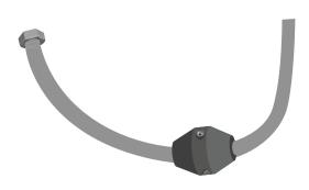
7. Connect the hand shower hose to its copper supply tube on the faucet, as shown. Insert the rubber O-ring into the lock nut before attaching. Apply a bit of thread sealant or plumber's tape to the threads before tightening. Hand tighten the connection, then finish tightening with a 1/4 turn using an adjustable wrench.
