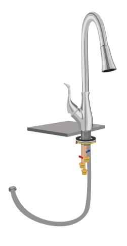
4. Attach the provided braided water lines to the copper supply tubes on the faucet. Apply plumber's tape or thread sealant to the threads before tightening. Ensure that you are connecting the hot and cold lines appropriately. Hand tighten the connections, then finish tightening with a ¼ turn using an adjustable wrench.
