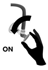
9. Remove the sprayer nozzle from the faucet by unthreading it from the hose. Turn the faucet on for approximately 60 seconds to remove any dust or loose sediment within the water lines, and to ensure that there are no leaks. Ensure that both hot and cold water are functioning properly. Reattach the sprayer nozzle and divert the water to the sprayer to ensure functionality.
