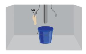
2. If the braided water lines came attached to the faucet, remove them by unthreading them from the copper supply tubes. Remove the lock nut, metal washer, and rubber washer from the faucet as well.
