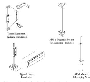
8. To remove the receiver from the machine, loosen the two clamps and remove the receiver from the mounting pipe. Be sure to store and transport the receiver in its carrying case.
