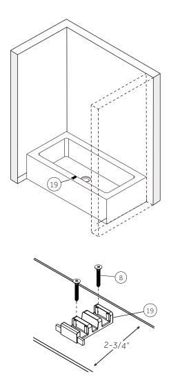
2. Disassemble the rail wall bracket kit (7) as shown. The mounting bracket kit (7) should be mounted 7/8" back from edge of door guide (19). The mounting bracket should be mounted 59-1/2" from the tub rim as shown. Drill installation hole with 1/4" drill bit. Apply a small amount of silicone sealant to the installation hole, then insert wall anchor (6). Attach rail wall bracket against the wall with 1-1/4" screw (8).
