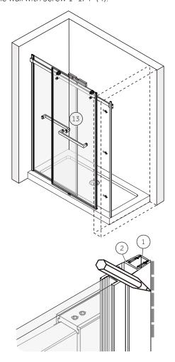
12. Note distance from wall to door guide (19), then cut threshold (16) to your noted distance less 1/2". Mark a hole for the threshold cover (15) for installation. Drill installation hole with 1/8" drill bit. Attach threshold cover (15) to tub rim with 1-1/4" screw (8).
