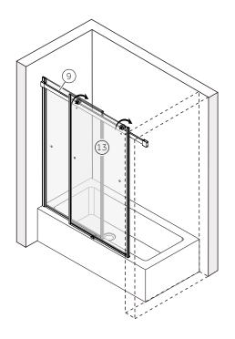
10. Install anti-jumper (12) on outer door (13). Install handle (5) on doors (3/13) as shown.
