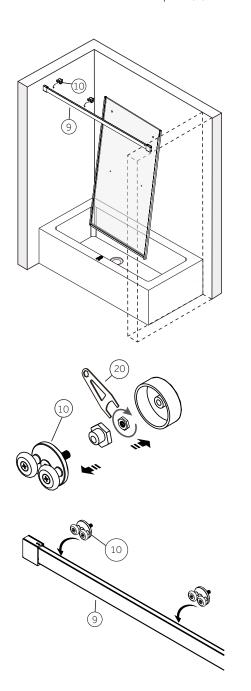
6. Insert inner door (3) onto the door guide (19) slot. Attach the inner door panel (3) to the top rail (9) with the double roller (10). Tighten the hexagonal nut with spanner (20).
