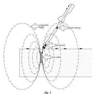
Sensor coils unbalanced by magnetic field of iron stake.
