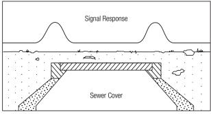
The joints, elbows and ends of iron pipes will create the strongest signals (*Fig. 8*). Hold the locator in a vertical position while searching to produce the best results.
