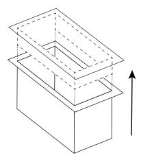
2. Insert the new floor register. The louver frame will fit into the air duct opening, while the lip of the register will sit on top of the floor. In general, it is not necessary to secure the register to the floor with screws or mounting clips.
