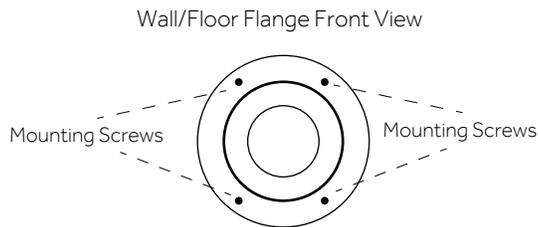
3. Drill mounting holes using the appropriate drill bit for the wall/floor surface or material.
