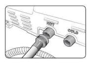
4. Connect the ends of the water supply hoses to the water supply intake connections at the back of the washer.
