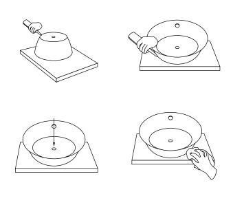
6. Let the assembled vanity sit for 24 hours to allow all the silicone sealant to fully dry. Once dry, proceed to the installation of your faucet and drain assemblies.
