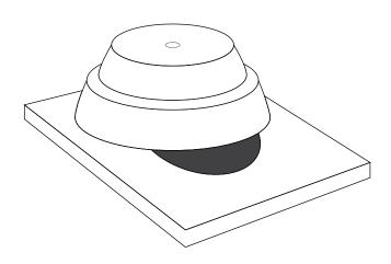
2. Apply a continuous bead of silicone sealant to the outer edge of the sink where it will contact the counter.
