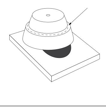
3. Turn the sink back over, placing it inside the sink's cutout and adjust the sink as necessary until centered. Once in position, press the sink firmly into place.
