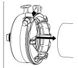
**Step 4** • With the bolt in the extended position, place the end cap onto the pipe end until the pipe makes contact with the inside of the end cap.
