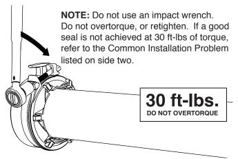
**Step 7** • Confirm proper installation by pressurizing the line and checking for leaks.
