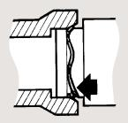
A bell not lubricated or improperly lubricated may cause gasket to roll and possibly damage the bell.
