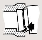
Improperly prepared spigot and gasket recess may prevent gasket from sealing correctly.
