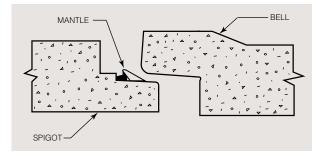
Step 2: Place self lubricating gasket on the spigot end of the joint, with the mantle (tube) towards end of spigot. The gasket must be seated against the spigot shoulder. Please note that no equalization of the gasket is required
