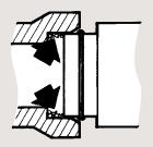
Improperly prepared bell jointing surface may prevent homing of the pipe.
