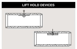
When pipe is provided with lifting holes, the lifting device should pass through the wall and distribute the weight along the inside barrel of pipe.
