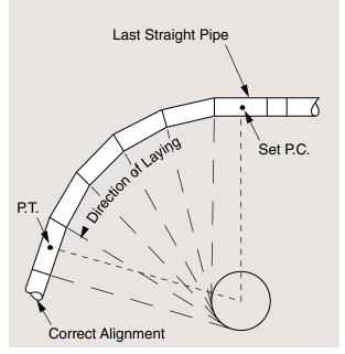
Special precast sections can be used for extremely short radius curves which cannot be negotiated with either deflected straight pipe or with conventional radius pipe. Sharper curves can be handled by using special short lengths of radius pipe rather than standard lengths.
