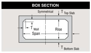
and Sewers with Less than 2 ft. (0.6 m) of Cover: Covers reinforced concrete box sections in 42 standard sizes and shapes under less than 2 ft. (0.6 m) of earth cover for two loading conditions; HS20 truck plus dead load, and alternate interstate loading plus dead load.
