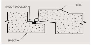
Step 3: Align the spigot with the bell and home the joint. When applying the homing force ensure the pipes are level to each other and the spigot section is not tilted and "rolled" into the bell. When the joint is homed, the mantle (tube) section slides over the compression area of the gasket and comes to rest on the spigot shoulder.
