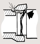
Excess force will be required to push the pipe to the home position if gasket is not well lubricated.
