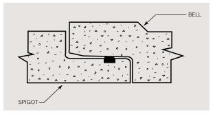
Step 5: Align the spigot with the bell ensuring that the gasket is in contact with the flared end of the bell around the complete circumference of the pipe, and apply a uniform force to home the joint.
