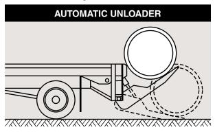
Unloading of the pipe should be controlled so as not to collide with the other pipe sections or fittings, and care should be taken to avoid chipping or spalling, especially to the spigots and bells. Caution should be exercised to be sure personnel are out of the path of the pipe as it is lowered. If the pipe has to be moved after unloading, the sections should be rolled or lifted and should never be dragged. Pipe sections should not be rolled over rough or rocky ground.
