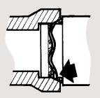
Improper alignment can dislodged gasket causing leaks or possibly break the bell.
