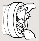
Carefully clean all dirt and foreign substances from the jointing surface of the bell or groove end of pipe.
