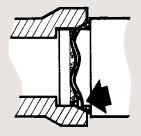
Improper alignment can dislodged gasket causing leaks or possibly break the bell.
