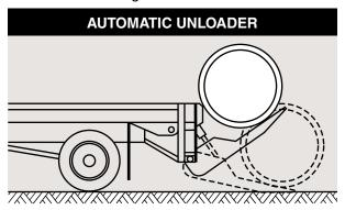
Unloading of the pipe should be controlled so as not to collide with the other pipe sections or fittings, and care should be taken to avoid chipping or spalling, especially to the spigots and bells. Caution should be exercised to be sure personnel are out of the path of the pipe as it is lowered.
