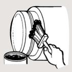
Lubricate the spigot or tongue end of pipe, especially the gasket recess.
