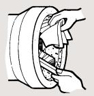
Carefully clean all dirt and foreign substances from the jointing surface of the bell or groove end of pipe.
