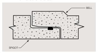
Step 5: Align the spigot with the bell ensuring that the gasket is in contact with the flared end of the bell around the complete circumference of the pipe, and apply a uniform force to home the joint.
