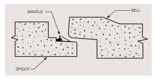
Step 2: Place self lubricating gasket on the spigot end of the joint, with the mantle (tube) towards end of spigot. The gasket must be seated against the spigot shoulder. Please note that no equalization of the gasket is required
