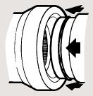
Align bell and spigot of pipes to be jointed. Before homing the joint, check that the gasket is in contact with the entry taper around the entire circumference.
