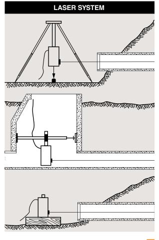
ordinary rule or stadia rod can measure offsets for construction quickly and accurately, generally within 1/16 in. (1.58 mm) or less. The laser instrument can be mounted in a manhole, set on a tripod or placed on a solid surface to project the light beam either inside or outside the pipe.
