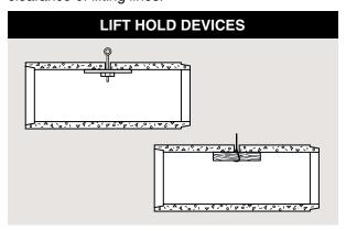
When pipe is provided with lifting holes, the lifting device should pass through the wall and distribute the weight along the inside barrel of pipe.
