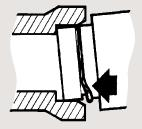
Improperly prepared spigot and gasket recess may prevent gasket from sealing correctly.
