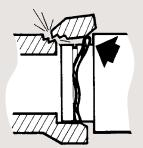
Excess force will be required to push the pipe to the home position if gasket is not well lubricated.
