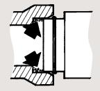
Improperly prepared bell jointing surface may prevent homing of the pipe.
