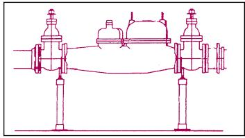
The Standon Support is ideal for use on backflow devices and large water meters. It is perfect for retrofitting existing installations, replacing ill fitting concrete blocks etc.
