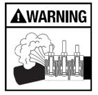
THIS PRODUCT DOES NOT RESTRAIN PIPE MOVEMENT. Proper anchoring is required to prevent pipe pullout. Failure to anchor or improper anchoring can result in dangerous pipe content escape, property damage, serious injury, or death. Read the product installation instructions prior to installing this product.
