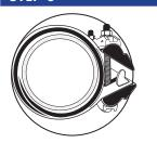
Once the HYMAX Clamp is positioned around the pipe, re-engage the side compression beam over the lug assembly by pushing it downward until it clicks in place TWICE.
