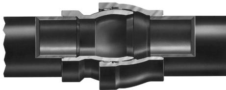
The AMERICAN Flex-Lok Joint, furnished in sizes 30"-60", is a boltless, very flexible joint. This joint is designed to provide up to 15° joint deflection for subaqueous or other difficult installations. Contact AMERICAN for 64" size requirements.
