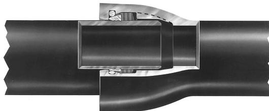
The AMERICAN Fast-Grip Gasket furnished in sizes 4"-30" provides flexible, field-adaptable joint restraint in a standard AMERICAN Fastite (or Flex-Ring) Bell. See Sections 4 and 9.
