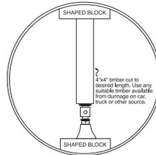
Note: Field rounding operations should be conducted without backfill on any part of large-diameter pipes and prior to encasing any part of pipe in concrete. If the inside of the pipe cannot be accessed to remove jacking materials, pipe ends can alternatively be rounded using external clamping means.
