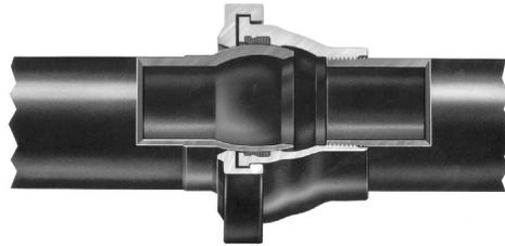
The AMERICAN Flex-Lok Joint, furnished in sizes 4"-24", is a boltless, very flexible joint. This joint is designed to provide up to 15° joint deflection for subaqueous or other difficult installations.
