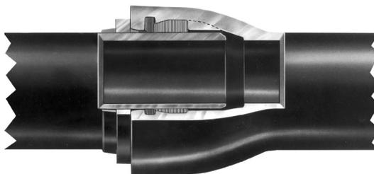
AMERICAN Fastite Joint Push-Bar pipe, furnished in sizes 4"-64", allows the AMERICAN Fastite Joint to be used in trenchless installations using direct jacking or pushing (including high load installations such as microtunneling and some pipe bursting applications). See Section 7.
