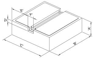
Maximum Load: 150 lbs. (Fig. 7715) 300 lbs. (Figure 7730) Height: 4 inches
