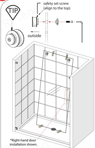
Before installing the **Panel Glass (#02)**, attach the two **Roller Assemblies (#04)** to the **Door Glass (#05)** with the wheels facing outside of the shower. Align the **safety set screw** towards the top for easier access. Then, take the **Door Glass (#05)** into the shower area and lean it against the wall with the handle holes on the correct side. Always use padding to protect the glass and shower surfaces.
