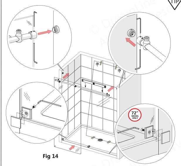
Adjust the installed **Top Guide Rail (#03)** to level as necessary using the **Guide Rail Brackets (#08)** first and then the **Glass-to-Rail Brackets (#07)**. **Start adjustments from the door end.**
