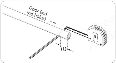
Model Width (-) Finished Opening (W) = Cut-off Length (L)
