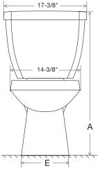
Note: All dimensions and specifications are nominal and may vary: Dimensions of 8" and greater have a tolerances of +3%. Dimensions less than 8" have a tolerances of +5%.
