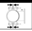
THIS PRODUCT REQUIRES UNIFORM TORQUE TO PROVIDE AN EFFECTIVE SEAL AGAINST THE PIPE SURFACE. Gap distances between product halves must remain equal while product is installed. The product must be evenly tightened across the sleeve to the required torque. The product will not function properly if the nuts on only the topside of the tapping sleeve are tightened. Failure to uniformly torque the product may cause damage to the pipe, sleeve, or result in product failure
