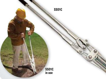
Reed's Standing Shut-Off Tool compresses 3/4" to 1" PE plastic tubes to stop the flow of water. The shut-off tool uses 30" handles to develop a clamping force in a manner similar to a pair of bolt cutters. The long handles make for easy shut-off from above the ditch with a chain (not included\*) to hold the tool closed. Not intended for gas service lines.
