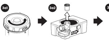
Rotate flow control cartidge counter-clockwise to release and remove from inlet diffuser
