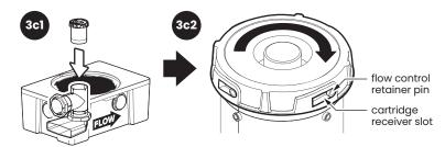
Slide flow control cartridge into top of inlet diffuser and rotate clockwise until cartridge drops onto flow control retainer pins. Continue rotating clockwise until pins are fully seated.
