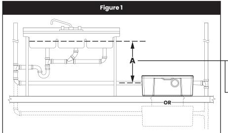
**Note to Plumbing Inspector** This interceptor includes certified internal flow control and does not require a dedicated "Flow Control Vent" (air intake).
