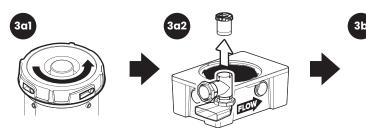
Rotate flow control cartidge counter-clockwise to release and remove from inlet diffuser
