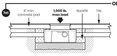
**Below Grade with Riser (preferred):** See instructions included with FCRI riser. Backfill evenly around tank using crushed aggregate (approximately 3/4" size rock or sand, with no fines), finish with a minimum 4" thick concrete pad.
