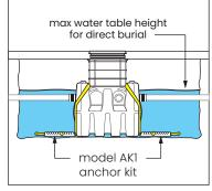
risk areas include but are not limited to tidal surge areas, floodplains and areas that receive storm water. Great Basin™ models that are direct buried in high water table scenarios must be installed with an anchor kit. Model GB-75 uses model AK1 anchor kit.
