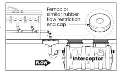
See drawing for guidance. For detailed guidance on indirect connections, go to:
