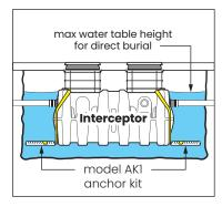
areas, floodplains and areas that receive storm water. Great Basin™ models that are direct buried in high water table scenarios must be installed with an anchor kit. Models GB-50, GB-75, and GB-250 use model AK1 anchor kit. Model GB-500 uses model AK2 anchor kit for use with deadmen anchors. Models GB-1000, GGI-750 and GGI-1500 use model AK3 anchor kit for use with deadmen anchors.
