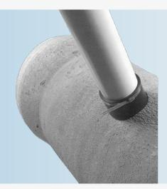
The Kor-N-Tee Pipe-to-Pipe Connector is an economical, watertight seal for concrete pipe that can be installed quickly and easily without complete excavation of the pipe and disruption of the bedding.
