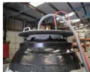
RISER-WRAP® VACUUM TEST
