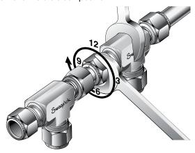
For 1/16, 1/8, and 3/16 in.; 2, 3, and 4 mm tube fittings, tighten the nut three-quarters turn to the 3 o'clock position.
