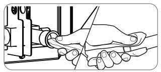
• Clean the inside of the fittings and outside of the tubing with a clean, dry cloth before soldering. Clean out debris, chips, dirt, etc., that enters tubing or service valve connections.
