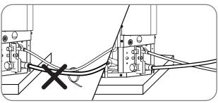
• Do not allow the bare suction line and liquid line to be in contact with each other. This causes an undesirable heat transfer resulting in capacity loss and increased power consumption.
