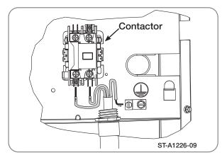
Connect power wiring to the line-voltage lugs on the contactor located in the unit electrical box. (See wiring diagram attached to unit access panel and above illustration.)
