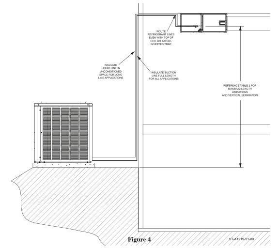
For applications that are considered to have a long line set with the outdoor unit below the indoor unit the following is required:
