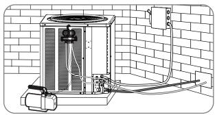
After the system has been leak-checked and proven sealed, connect the vacuum pump and evacuate system to 500 microns and hold 500 microns or less for at least 15 minutes. The vacuum pump must be connected to both the high and low sides of the system by connecting to the two pressure ports. Use the largest size connections available since restrictive service connections may lead to false readings because of pressure drop through the fittings.
