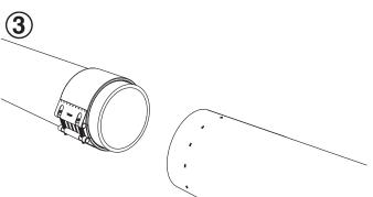
Step 4 • Bring the other pipe end to a facing position. Make sure the pipes are aligned concentrically and that both pipe ends are correctly supported. See tolerances indicated on the label.
