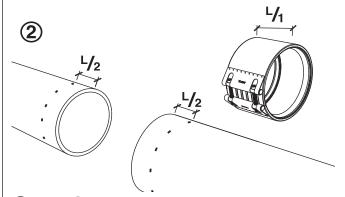
Step 3 • Without opening the coupling, slide the coupling over one pipe end.
