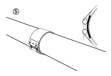
**Step 6** • Do not rotate the coupling or the pipe during tightening. Tighten the bolts alternately and evenly to the required torque. If there are three bolts, start with the center bolt, and begin tightening.
