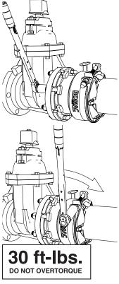
**Step 6** • Bring the mating flange into position and assemble the flange joint using the flange bolts. Be sure to maintain proper pipe insertion described in Step 4.
