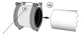
Connector for cathodic protection.
