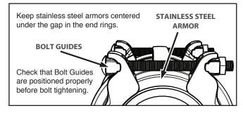
**Step 5** • Tighten each bolt until the gasket contacts the pipe and the coupling is snugly held in place. This should happen at approximately 10 - 20 ft-lbs.
