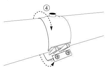
**Step 5** • Slide lifter bar up the receiver lug profile and snap into place over the sidebar edge. Confirm that the gasket is aligned in its pocket.
