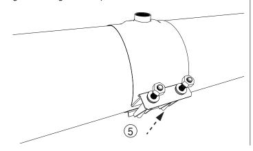
**Step 6** • Tighten all nuts evenly in 20 ft-lbs. increments. Use a wrench with at least a 12 inch handle. Close all gaps between the shell and the pipe surface evenly, and torque according to specifications below. Bolt resistance will increase guickly once the saddle is properly installed.
