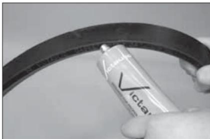
**4. CHECK GASKET AND LUBRICATE:** Check the gasket to make sure it is suitable for the intended service. Apply a thin coat of Victaulic Lubricant or silicone lubricant to the gasket lips and exterior. **NOTE:** This gasket is designed to provide the sole seal. However, reference should be made to the notes at the beginning of this section for special applications.
