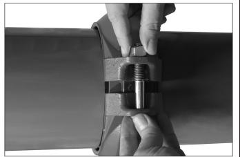
4. INSTALL HOUSINGS: Install the housings over the gasket. Verify that the housings' keys engage the grooves completely on both mating components.
