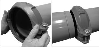
**5. ASSEMBLE JOINT:** Assemble the joint by inserting the grooved end of a CPVC/PVC mating component into each opening of the coupling. The ends of the grooved mating components shall be inserted into the coupling until contact with the center leg of the gasket occurs. A visual check is required to verify that the coupling keys align with the grooves in the mating components. **NOTE:** The coupling may be rotated to verify that the gasket is seated properly.
