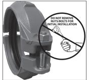
1. DO NOT DISASSEMBLE THE COUPLING: Style 357 Installation-Ready<sup>™</sup> Rigid Couplings are designed so that the installer does not need to remove the bolts and nuts for installation. This design facilitates installation by allowing the installer to directly insert the grooved end of mating components into the coupling.
