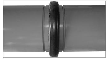
3. JOIN MATING COMPONENTS: Align the two grooved mating component ends. Insert the other mating component end into the gasket until it contacts the center leg of the gasket. NOTE: Verify that no portion of the gasket extends into the groove of either mating component.
