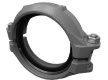
• METHOD 1 FOR REASSEMBLY: The coupling can be reassembled into its "installation-ready" condition by installing the gasket into the housings, then inserting the bolts and threading a nut onto each bolt until 2 – 3 threads are exposed, as shown above. If this method is chosen, steps 1 – 3 in the left column, along with all steps on page 2, shall be followed.
