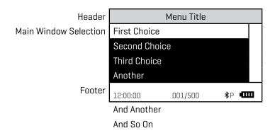
A light bar will indicate the menu choice. As the menu is scrolled through, the light bar will highlight different menu choices. Pressing the button will select the menu choice that is indicated by the light bar.
