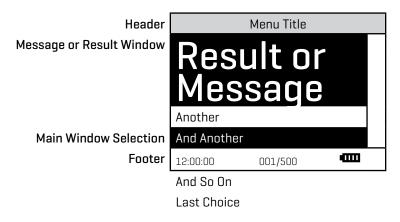
As described previously, the two button allows an exit or escape from the current menu and a return to the previous menu. This allows a rapid exit from an inner menu to the main menu by repeatedly pushing the two button. Pushing the time will turn the colorimeter off.
