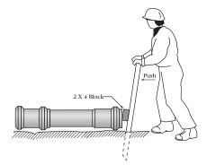
Multi gasketed sewer fittings can normally be assembled by hand or by bar and block for sizes up to 15". For larger sizes, it may be necessary to install the pipe using methods such as lever pullers, hydraulic jacks or the backhoe bucket.
