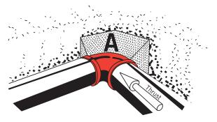
area A = <u>Thrust Force</u> Bearing Strength of Soil
