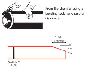
Apply a thin coating of lubricant (about 1/32" thick, equivalent to a brushed coating) using a glove, a rag, or a paint brush. The area to be covered is as follows:
