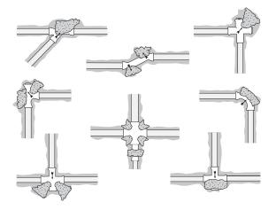
Typical thrust block locations. Trim the trench bearing area using hand tools to be sure of undisturbed soil.
