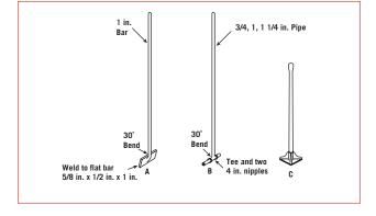
**Tampers** - These devices are well-suited for use in the Bedding, Haunch, Initial Backfill, or Final Backfill zones. A minimum cover of 12" is recommended for jumping jacks to avoid excessive impacts, while flat plate tampers may be used with as little as 6" of backfill over the pipe and fittings.
