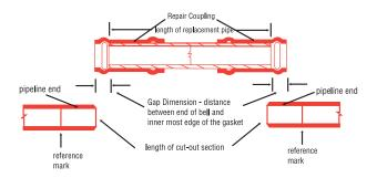
When cutting out the section be sure that all the damage is included (ie.) no hairline fractures are left in the line and that there is enough room to carry out the repairs.
