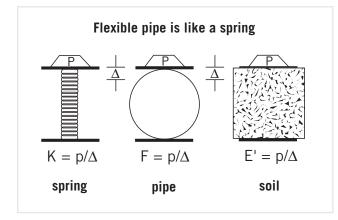
The ability to deflect away from vertical load is what gives PVC pipe its load carrying capability. The arching action of the soil over the pipe tends to reduce the load on the conduit, while the load that is applied is transferred to the surrounding bedding.
