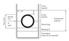
Foundation - A foundation is required when the trench bottom is unstable. Any foundation that will support a rigid pipe without causing loss of grade or structural breakage will be more than adequate for PVC pipes.
