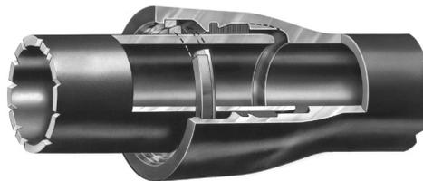
The AMERICAN Flex-Ring Joint provides flexible joint restraint against thrust due to internal water working pressure or external forces. It is also used in horizontal directional drilling (HDD) and pipe bursting applications. See Sections 4 and 9.
