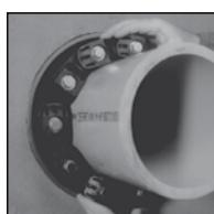
**Installation Notes:** The LINK-SEAL® modular seal bolt heads are usually recessed below the wall opening or the edge of casing pipe and therefore a socket or offset wrench must be used.
