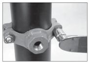
5. TIGHTEN NUTS: Make sure the locating collar is still positioned properly in the outlet hole. Tighten the nuts evenly by alternating sides until the upper (outlet) housing contacts the pipe completely.
