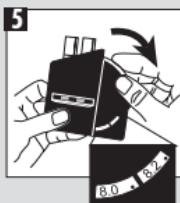
The mirror unit makes use of the view through the entire length of the cuvette. Compare the two colour fields and ⑩ read off the result as total chlorine in mg/l.
