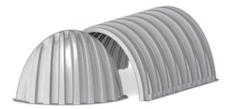
With all StormTech chambers, one chamber type is used for the start, middle and end of rows. Rows are formed by overlapping the upper joint corrugation of the next chamber over the lower joint corrugation of the previous chamber **(Figure 6)**.
