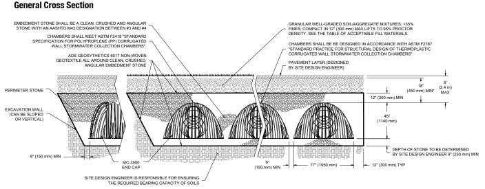
\*MINIMUM COVER TO BOTTOM OF FLEXIBLE PAVEMENT. FOR UNPAVED INSTALLATIONS WHERE RUTTING FROM VEHICLES MAY OCCUR, INCREASE COVER TO 24" (600 mm).
