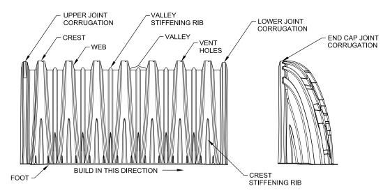
FIGURE 6—Chamber Joint Overlap
