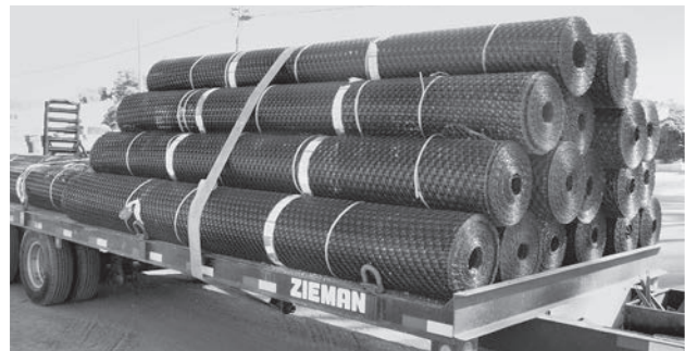
Storing the Tensar Geogrid rolls horizontally.
