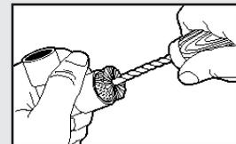
4. Apply flux thoroughly to inside of fitting.
