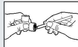
5. Apply flux thoroughly to outside of tube—assemble tube and fitting.
