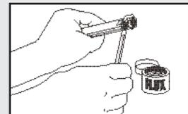
6. Apply heat with torch. When solder melts upon contact with heated fitting, the proper temperature for soldering has been reached. Remove flame and feed solder to the joint at one or two points until a ring of solder appears at the end of the fitting.
