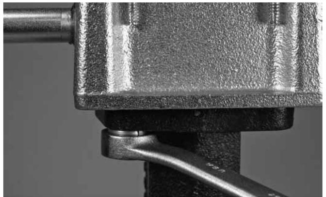
8. Use the hex-head screws (Item 7) and lock washers (Item 6), removed in Step 3, to secure the new gear operator to the valve body mounting flange. Tighten the hex-head screws until the lock washers are fully compressed.
