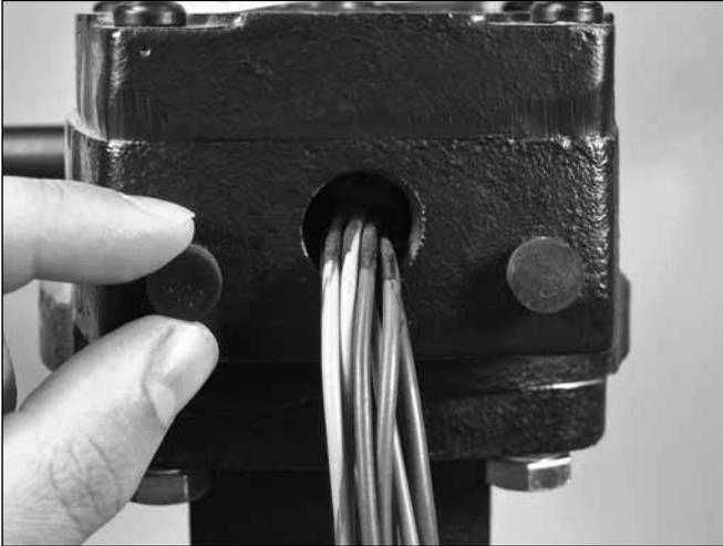
2. Remove the dust cap from the left side of the gear operator.
