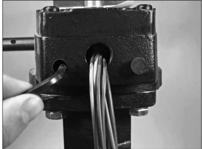
4. With the valve disc in the desired open position, tighten the internal set screw (clockwise) with a  $\frac{1}{32}$  allen wrench.
