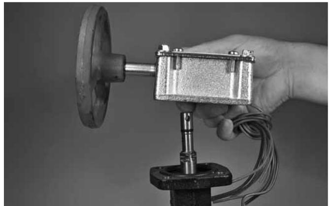
4. Lift the gear operator (Item 2) straight up off the valve body mounting flange. Use caution when removing the gear operator in order to prevent damage to the stem.
