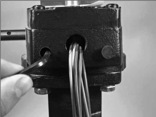
3. Using a  $\frac{1}{32}$  allen wrench, loosen the internal set screw counterclockwise.
