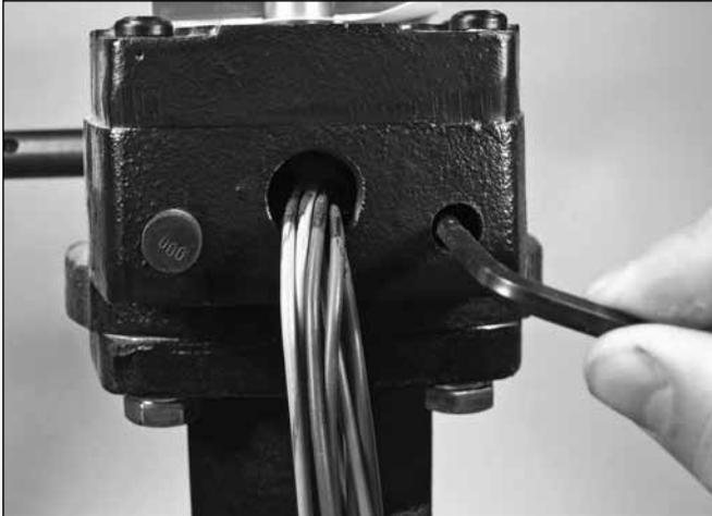
3. Using a  $\frac{5}{32}$  allen wrench, loosen the internal set screw counterclockwise to increase the distance for disc travel.
