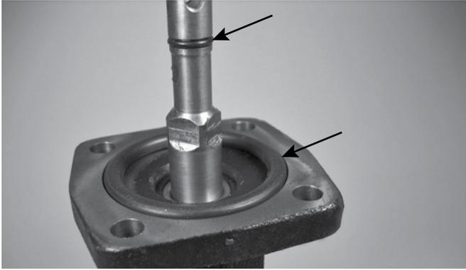
5. Inspect the o-ring between the gearbox and valve body mounting flange (Item 3) and the o-ring around the valve stem (Item 4) for signs of damage. Replace the o-rings, if necessary.
