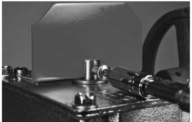
9. Re-install the actuator flag onto the valve stem with the self-tapping torx screw removed in Step 2.
