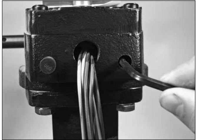
4. With the valve disc in the closed (shut) position, tighten the internal set screw (clockwise) with a  $\frac{5}{32}$  allen wrench.
