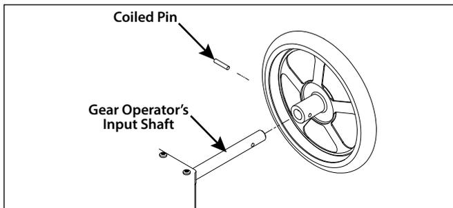
6. **FOR 10 - 12-INCH/273.0 - 323.9-MM VALVE SIZES:** The gear operator is shipped without the handwheel (Item 9) installed. Install the handwheel onto the gear operator's input shaft. Align the hole in the handwheel's hub with the input shaft's hole. Drive the coiled pin (Item 8) through the handwheel and input shaft.
