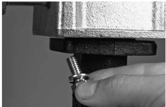
3. Remove the hex-head screws (Item 7) and lock washers (Item 6) from the underside of the gear operator (Item 2), where the gear operator mounts to the valve body mounting flange.
