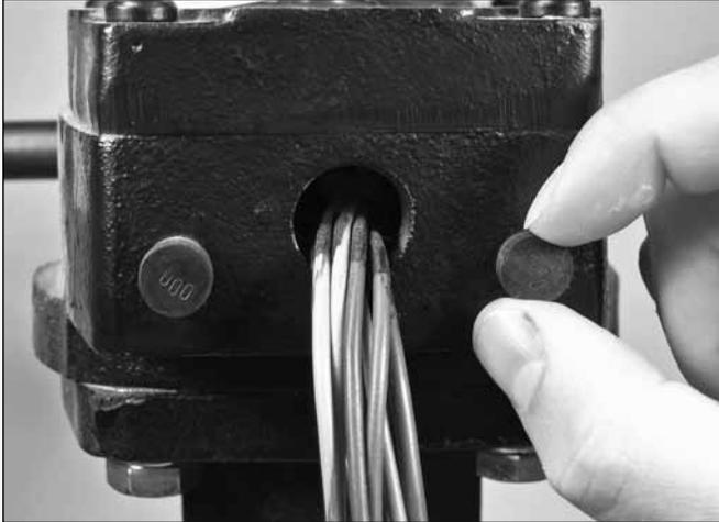
2. Remove the dust cap from the right side of the gear operator.
