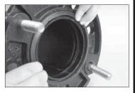
**5a.** Make sure the gasket is seated properly in the flange adapter.
