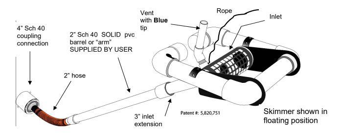
2. Glue the 8' long 2" sch 40 barrel to the 2" grey coupling on the hose.
